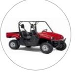
A utility terrain vehicle (UTV) has similar characteristics to an ROV but typically also features a box bed. UTVs are generally designed for utility rather than for recreational purposes.
